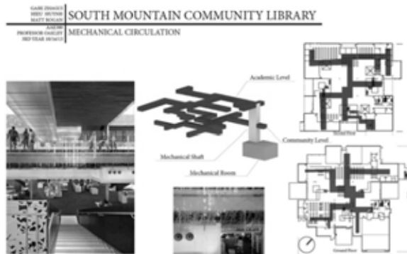
Fig. 3. Mechanical systems diagram for the South Mountain Community Library, generated by students based on published documents.
