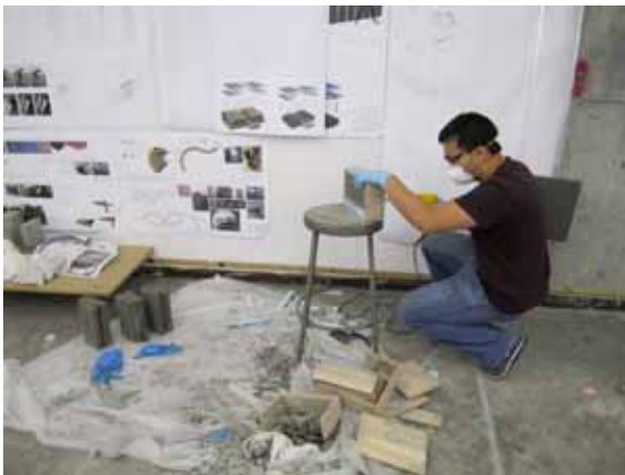
Figure 4. Disassembling formworks for concrete blocks (Materials workshop – Jonathan Arcila-Garcia)
