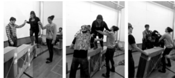
Fig. 5. A "live" load on a proposed Cardboard Catwalk
