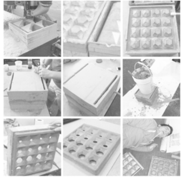
19_ Milled component mold process. student work
