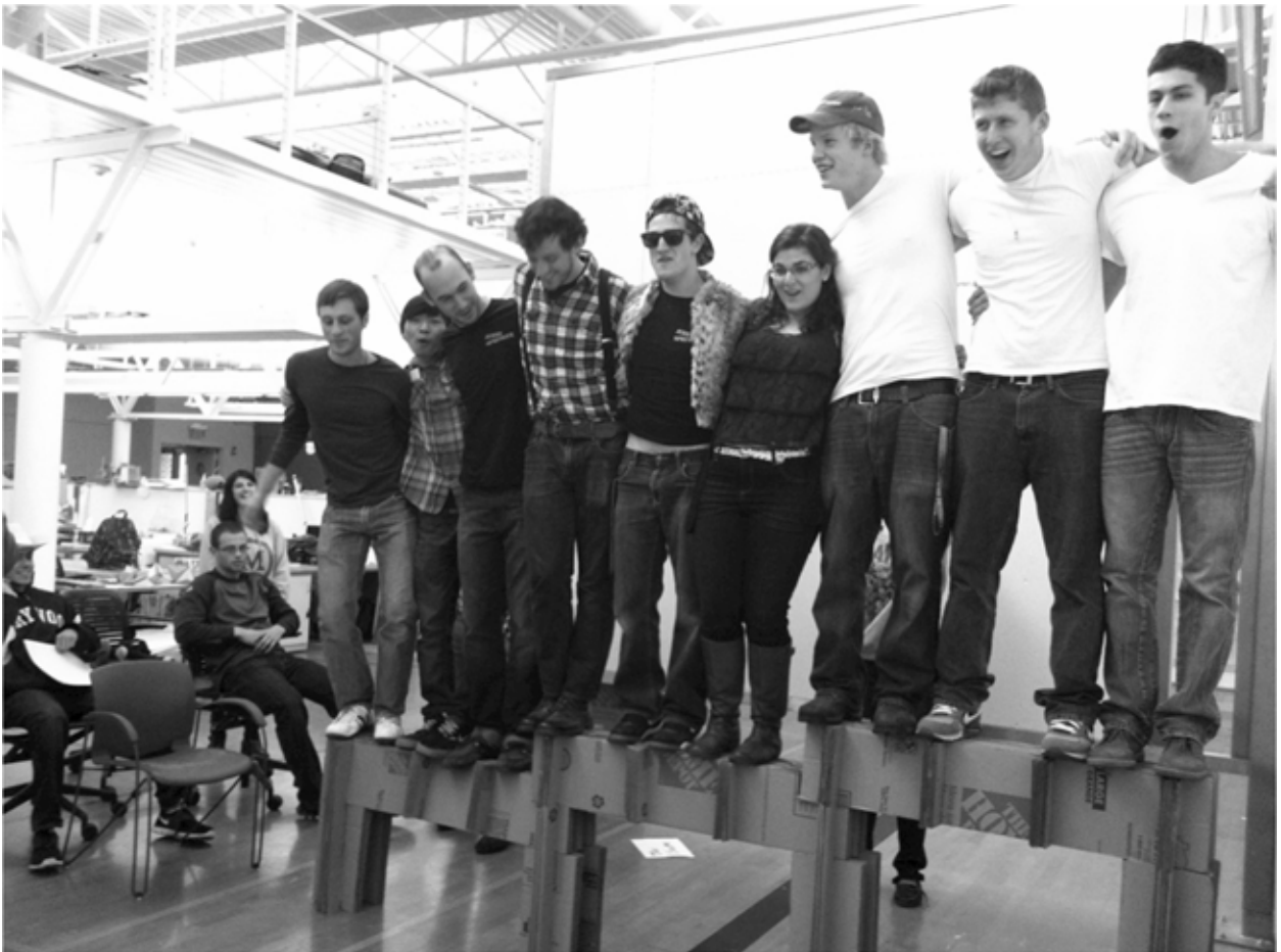
Fig. 6. A team of three students designed the only Cardboard Catwalk able to support nine "live" loads of appx. 1500lbs
