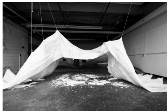
Fig. 11. Wax thin shell stood for 40 minutes before collapsing during final review. Students: C. Maier, N. St John, J. Ding, A. Tong, W. Van Deusen, Z. Boucetta. Photograph: G. Rafailidis.
