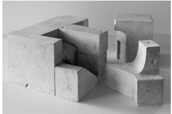
Fig. 4. Multi-part plaster mold with foam original. Student: J. Costello. Photograph: G. Rafailidis, 2012.
