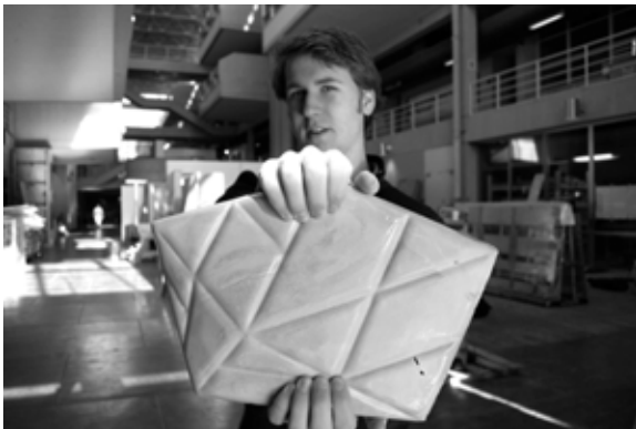
Fig. 3. Hollow Concrete Unit Prototype. Image: Author
